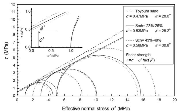
FIGURE 9. Shear strength and Mohr's circles of hydrate-bearing specimens.
