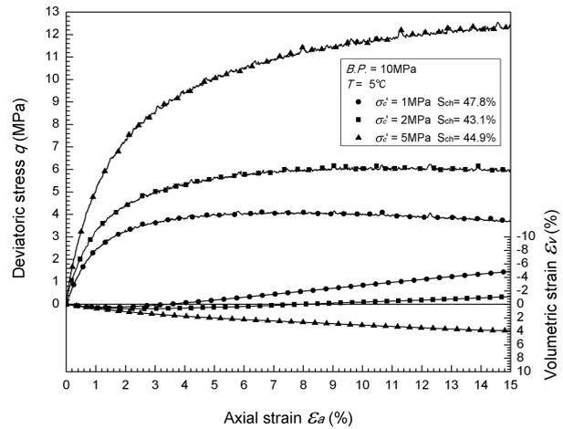
FIGURE 5. The influence of effective confining stress on the stress-strain curves and volumetric strain of carbon dioxide hydrate-bearing specimens.
