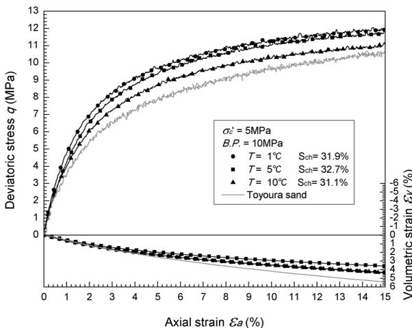
FIGURE 7. The influence of temperature on the stress-strain curves and volumetric strain of carbon dioxide hydrate-bearing specimens.
