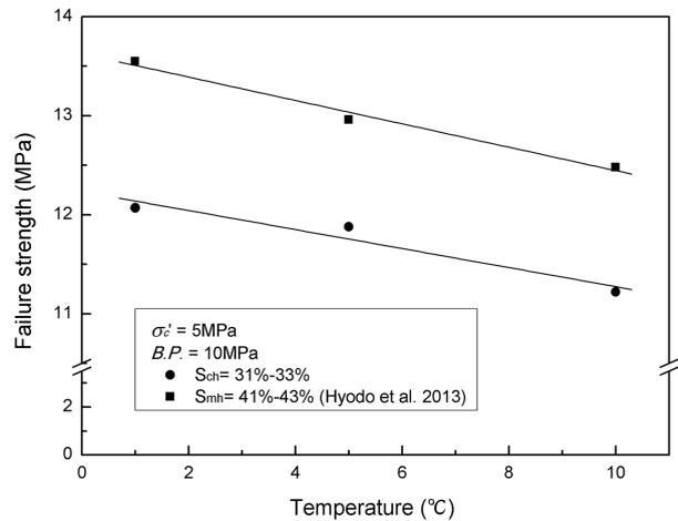
FIGURE 8. The influence of temperature on the failure strength of carbon dioxide and methane hydrate-bearing specimens.
