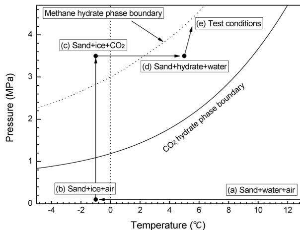
FIGURE 1. The pressure/temperature conditions during the preparation of carbon dioxide hydrate-bearing specimens.
