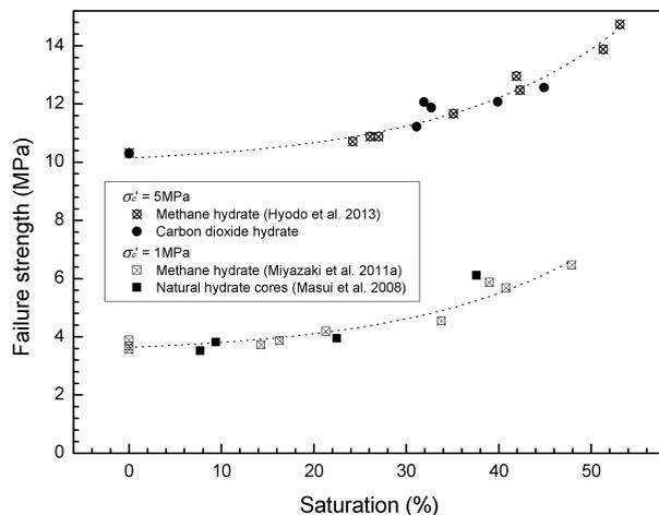
FIGURE 4. The influence of hydrate saturation on the failure strength of synthetic carbon dioxide hydrate, methane hydrate, and natural hydrate cores.
