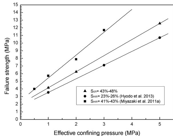
FIGURE 6. The influence of effective confining stress on the failure strength of carbon dioxide and methane hydrate-bearing specimens.
