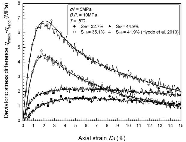
FIGURE 3. The deviatoric stress difference relative to the host Toyoura sand for various hydrate saturations under different hydrate saturation conditions.
