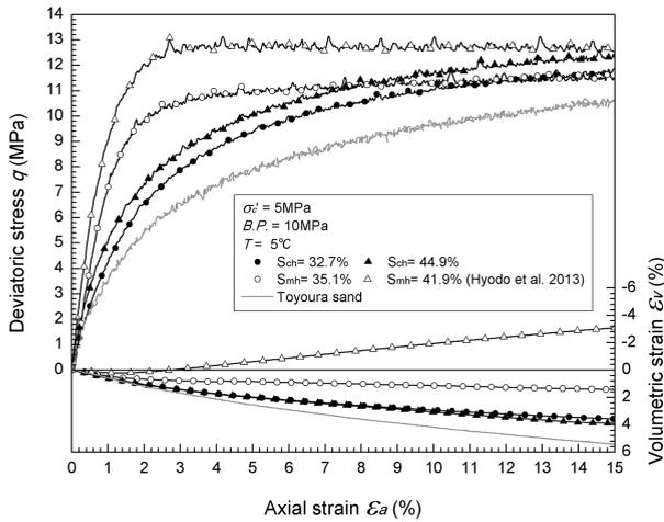
FIGURE 2. The stress-strain curves and volumetric strain of carbon dioxide and methane hydrate-bearing sediments.
